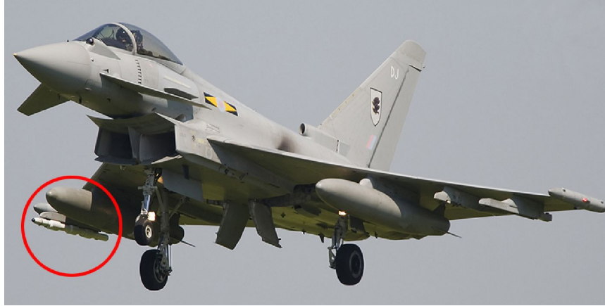
MBDA/MLM RAIDS (Rangeless Airborne Instrumented Debriefing System)
